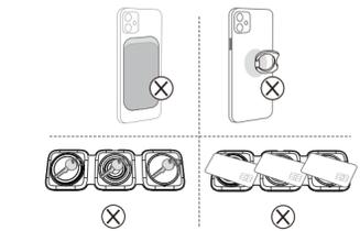
\*\*Thick protective case ≥ 5mm or a case includes magnet or metallic material, may not allow proper charging function.
